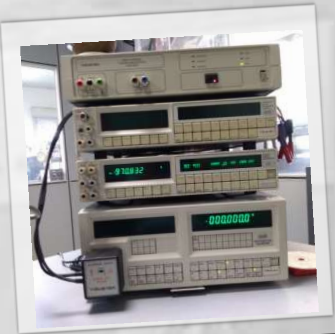
Automatic Calibration Station (Radio waves)
