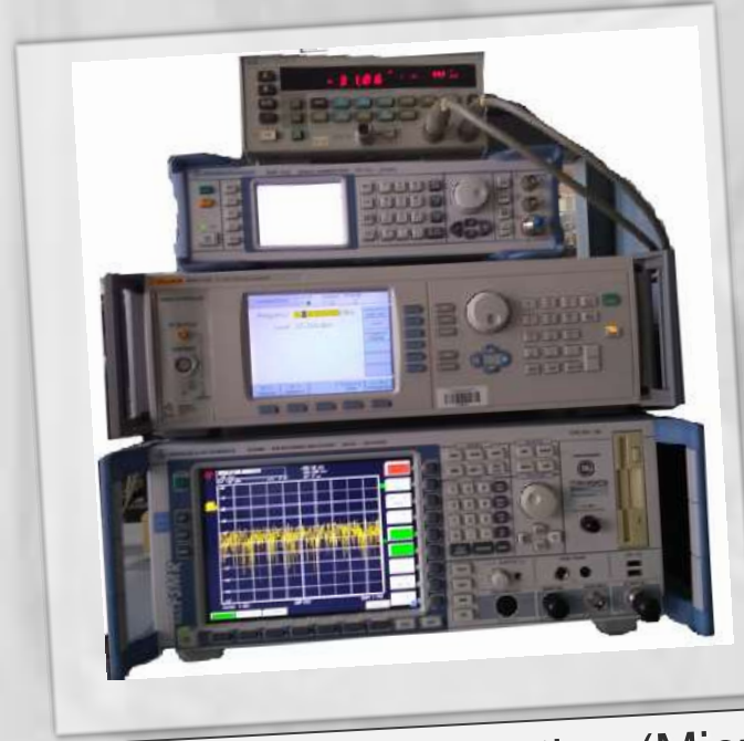
Automatic Calibration Station (Microwaves)
