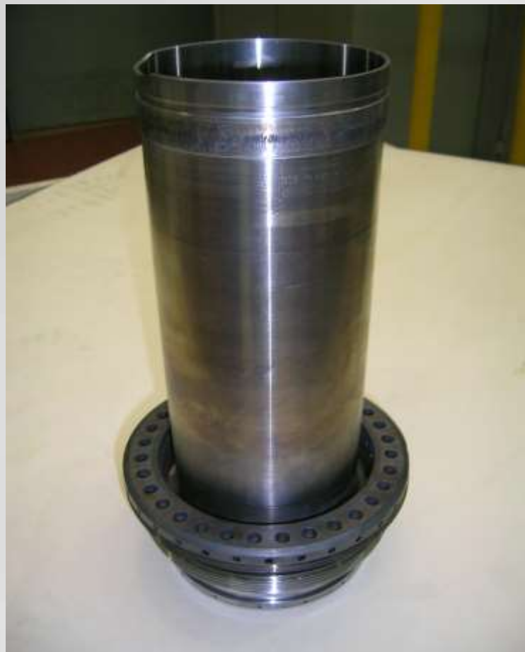
Concentricity checks of the HP turbine's PTO shaft installed on RB199 engine
